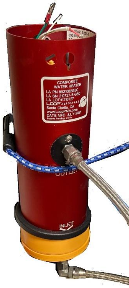
PRESSURE TEST SET-UP EXAMPLE FIGURE 5
